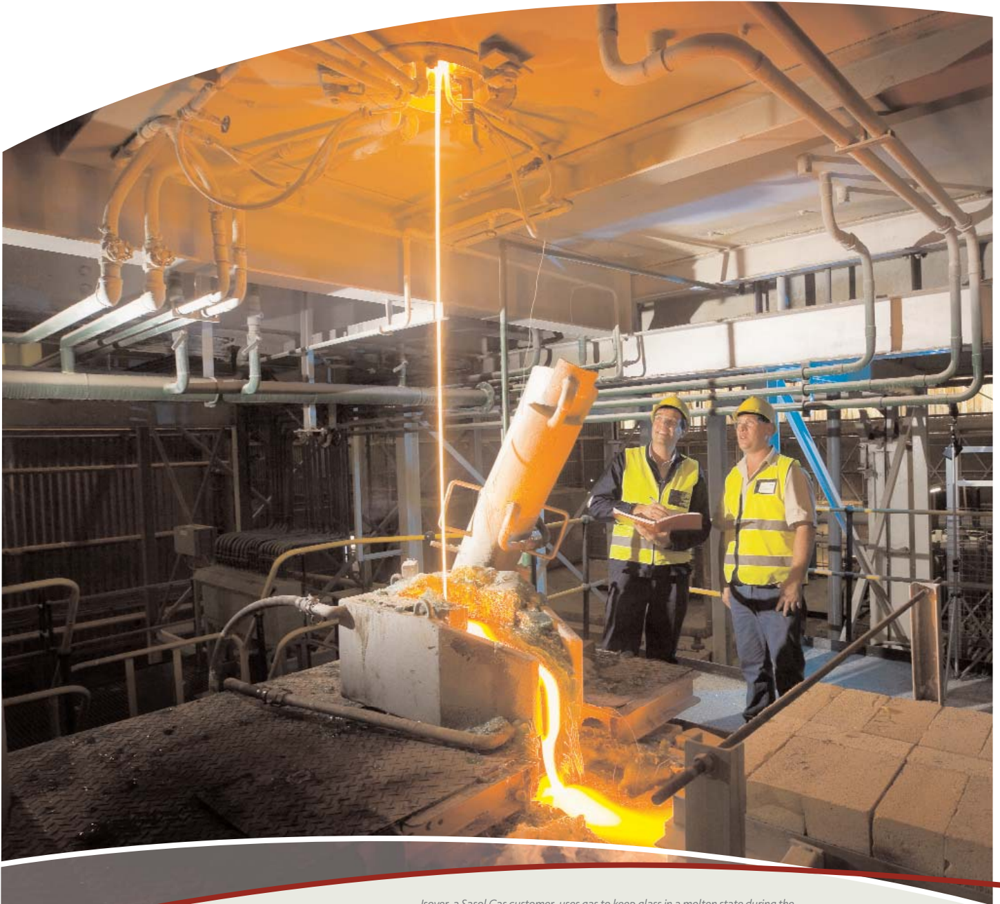
Isover, a Sasol Gas customer, uses gas to keep glass in a molten state during the manufacture of insulation fibreglass, at their plant in Springs.
