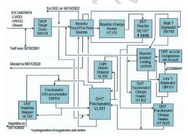
Figure 20: Distillate Hydrotreater (U35/235)
