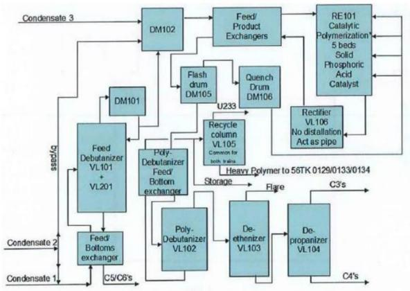
Figure 24: Catalytic Polymerisation and LPG Recovery (U32/232)
