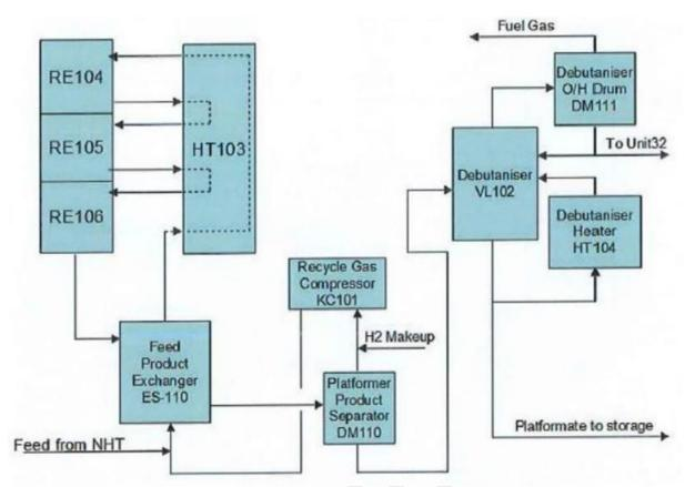
Figure 15: Naphtha Hydrotreater, Platformer and Continuous Catalyst Regeneration (Unit 30/230 & 31/331)
