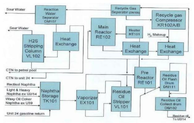
Figure 13: Coal Tar Naphtha Hydrogenation (U15/215)
