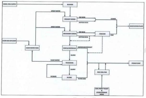
Figure 4: Coal Processing
