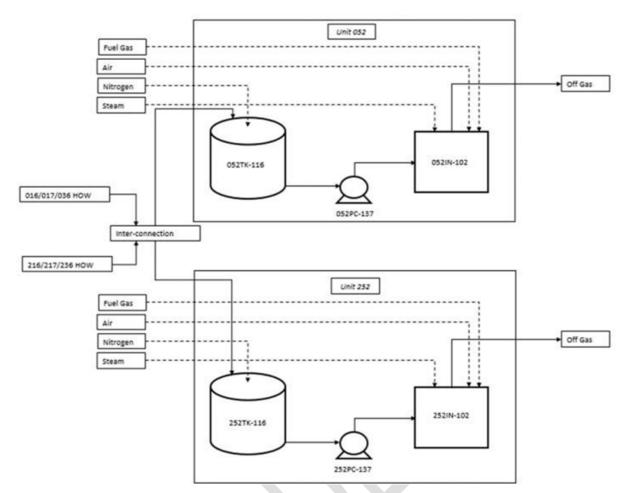
Figure 34: High Organic Waste (HOW) incinerators
