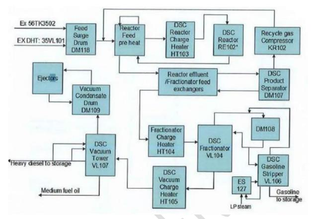
Figure 21: Distillate Selective Cracker (U35)
